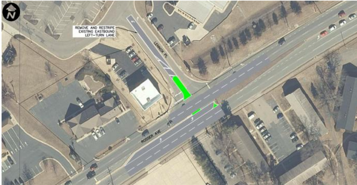
Figure 4: Rosser Avenue and Lennox Place Traffic Signal Removal
